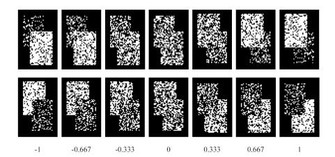
Figure 1: Snapshots of haptic stimuli. White points represent raised taxels, black dots represent lowered taxels. Numbers show the value of  $\lambda$ . The exact pattern of taxels changes each time the carriage is moved; only the probability of a taxel being raised in each rectangle is constant. For each value of  $\lambda$  there are two possible stimulus conformations.
